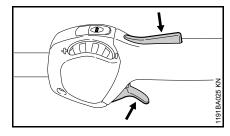
Depress throttle trigger lockout and pull the throttle trigger – the choke knob moves to the Run I position.
