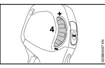
The throttle set wheel (4) enables the travel of the throttle trigger to be preset anywhere between idle and full throttle.
